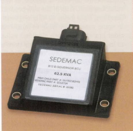
In the Econoseek system, an electronic reader board senses the electrical load
